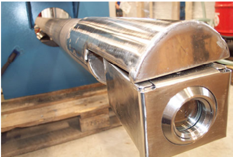
Camera head mounted to the traversing lance
